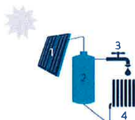
1 Zonnecollector | 2 Opslagvat zonnewater | 3 Sanitair warm water | 4 Radiator
