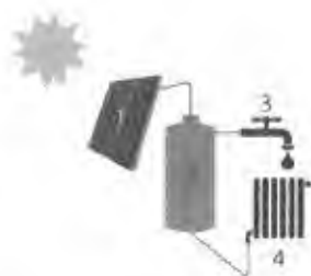
1 = Zonnecollector 2 = Opslagvat 3 = Sanitair warm water 4 = Radiator
